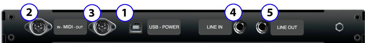
3. **Jack 3.5 mm MIDI OUT.** (3 pin) Tabletop / **DIN 1u Rack Module Version**
