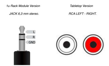
Sensibility AUDIO LINE LEVEL: 3.12 Volts p-p (in) 3.16 Volts p-p (out). -10db
